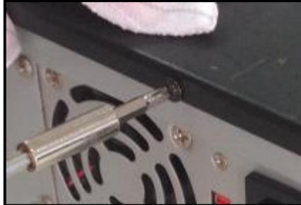
2. Fix the HDD in the case;
