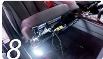
8 Another side of the LVDS cable should be brought to the front under the seat
