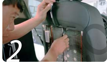
2 Check the location of the LVDS cable
