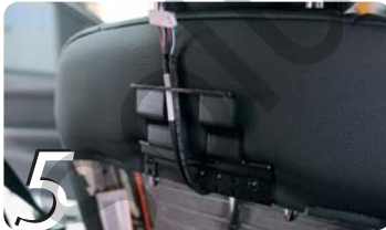
5 Pull out the cable through the hole of bracket
