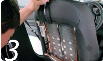
3 Cable should be arranged by using cable tie
