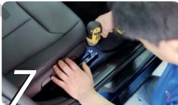
7 Loose the bolt in order to lift the seat
