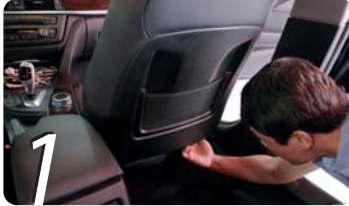
1 Remove the back cover from the seat
