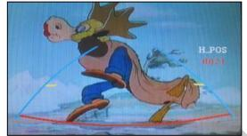
In H-POSITION, use  $\triangleleft$ ,  $\triangleright$  on remote control, to adjust parking guideline left and right.
