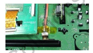
Put offered TOUCH OUT cable on the place where original touch cable was taken, put tape to make it fix.
