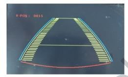
In V-POSITION use  $\triangle$ ,  $\nabla$  on remote control, to adjust parking guideline up and down.
