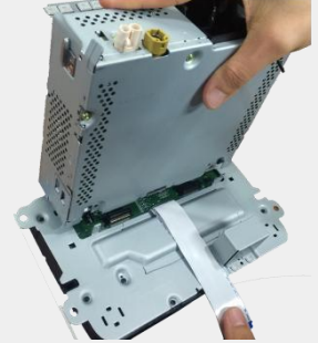
Reassemble the LCD part to the head unit with arranging cables as picture above.
