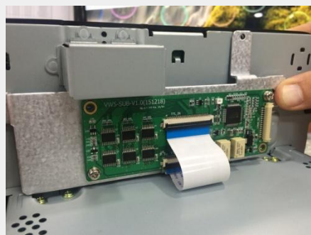
Assemble the sub-board and connect FFC cables
