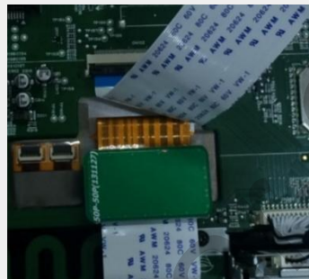
Disconnect the original FPC cable and connect it to Touch sub-board.
