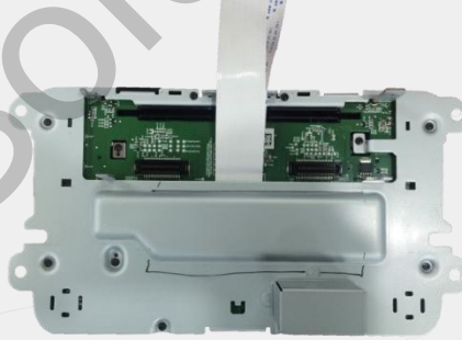
Connect the provided FFC cable #1 to the other side of Touch sub-board.
