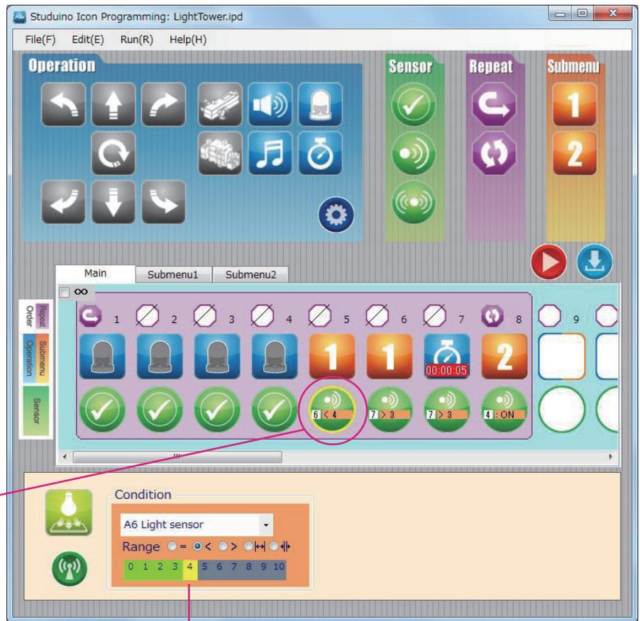
Click the Submenu 1 tab to calibrate the sensors and you will see a box to adjust the range settings.
