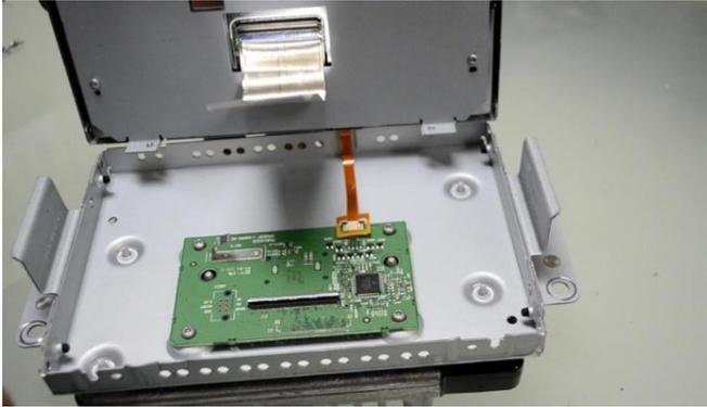
1) Please dismantle a monitor and disconnect LCD and cables.
