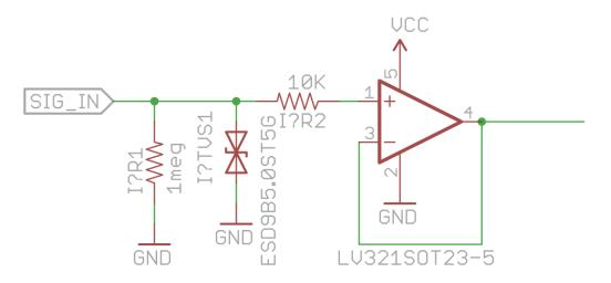
Figure 2: Example of an input stage, included in the Eagle templates
