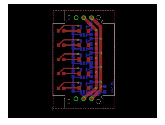
Figure 4: Example of neat component placement. Note how components are placed in line with each other.
