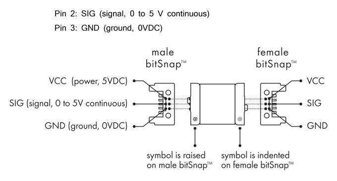
Figure 1: Male and female bitSnap™ connector pinouts
