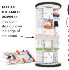
On both circuits, turn power on. On the **TRANSMITTER-CIRCUIT**, slide the dimmers to change the direction and speed of the wheels on your projector circuit. **TROUBLESHOOTING PG 20**
