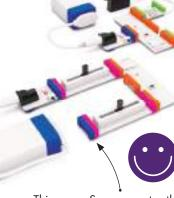
This powerSnap re-routes the power coming from the power Bit, so the circuit only needs one power Bit.
