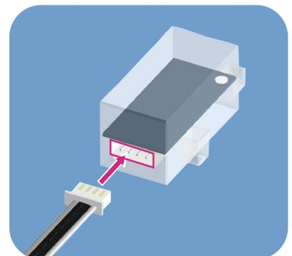
⚠ Make sure the cables are inserted correctly!
