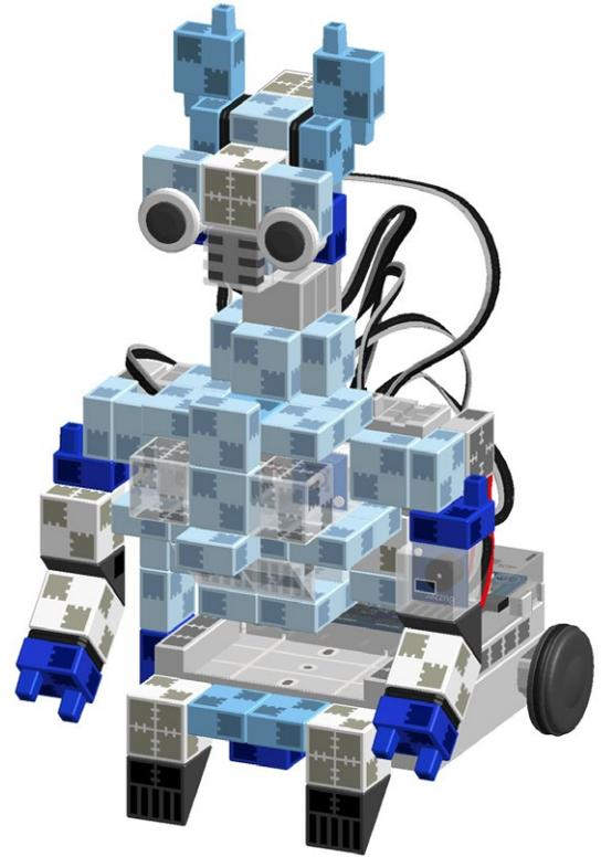
① Connect the cable from servomotor **D9** to its corresponding place on your Studuino unit.
