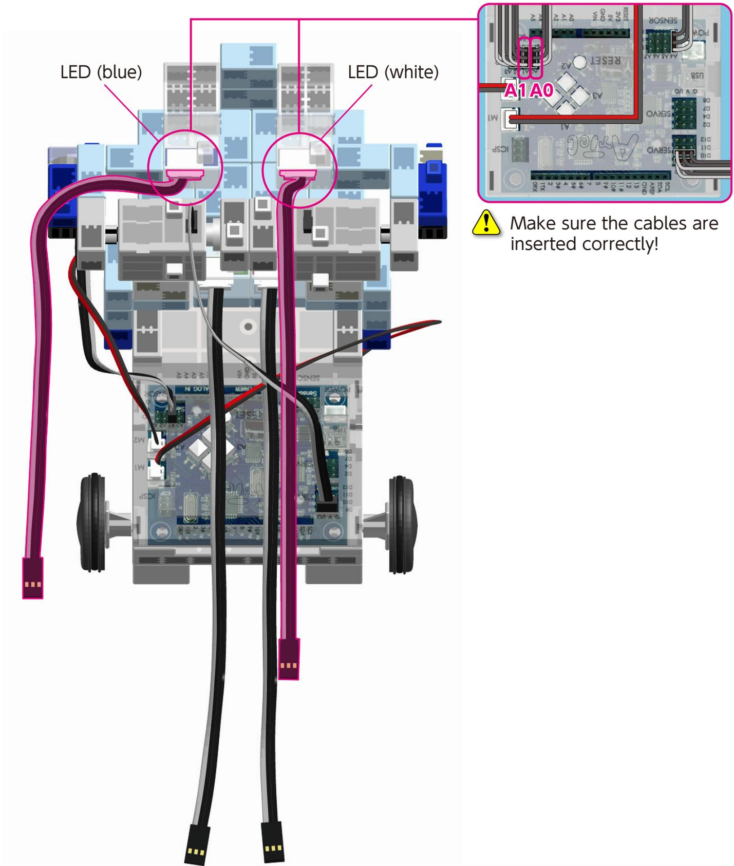
**!** Make sure the cables are inserted correctly!
