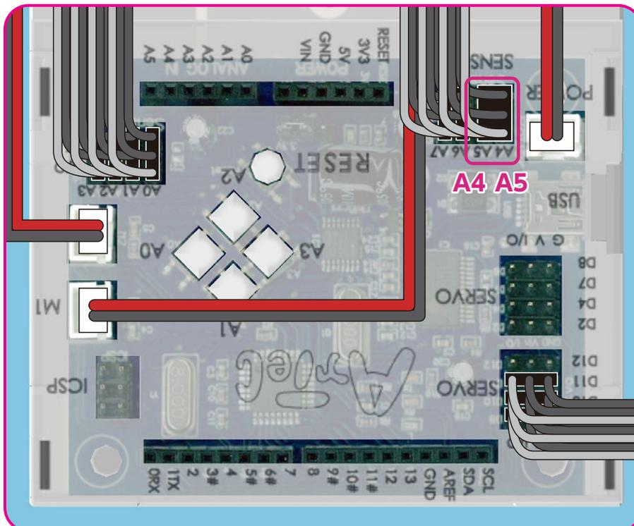
⚠ Connect to the accelerometer to both A4 and A5.
