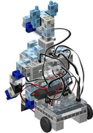
Connect the light sensor to the body and its cable to **A7**.
