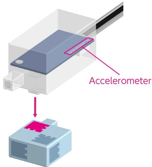
② Unplug the buzzer from **A4** and connect the accelerometer cable to **A4/A5**.
