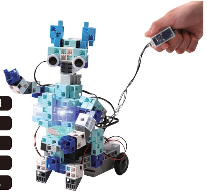
**!** Immediately turn the switch to off if your robot does not move as shown in the above picture when you tilt your accelerometer to the left. Not doing so may damage the servomotor.
