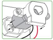
Using 2 screws, secure the motor by aligning the cover to the base.
