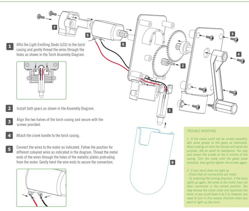
add some grease to the gears as lubricants. Most cooking oil from the kitchen will serve the purpose. Ask an adult for assistance. You may also loosen the screws at the 4 corners of the casing. Turn the crank until the gears move smoothly, then gently tighten the screws again.
