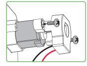
**8** Cover the LED with the transparent cover. Press gently until it fixes into place. Your very own Dynamo Torch is complete. Turn the crank in a clockwise direction and the torch will light up.
