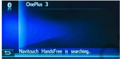
Choose a phone you would like to connect and press its name. The system will show 2 messages: one that indicates that the connection process has started and the other one that will provide you with a passkey you will need to enter to complete the connection process. A message will also appear on your phone, asking you to confirm the connection (for Android devices, the message will ask for access to contacts).
