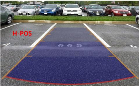
In H-POSITION, use ◀, ▶ on remote control, to adjust parking guideline left and right.
