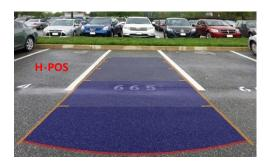
In H-POSITION, use  $\triangleleft$ ,  $\triangleright$  on remote control, to adjust parking guideline left and right.
