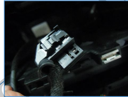
① Remove a harness from 12-pin connector.
