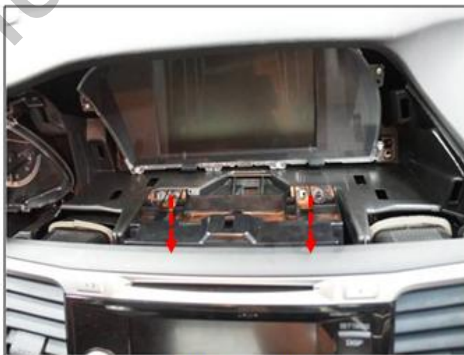
Pull out the Bolts
