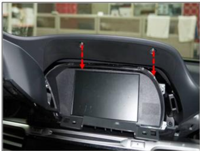
Pull out the Bolts
