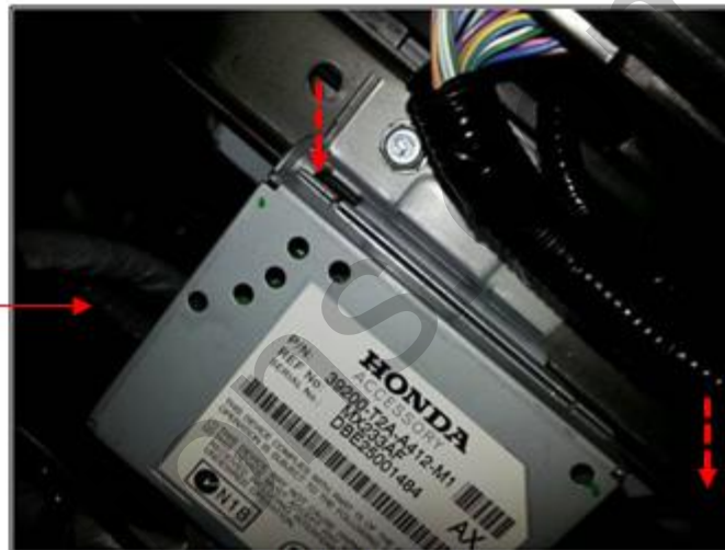
Pull out the Bolts
