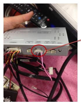
Connect one wire into the most right pin hole of RGB Out cable. It's Q-ROI RGB Uart wire.
