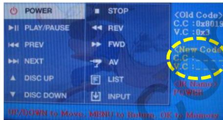
1. First of all, press ◀ button on remote controller 2 seconds long or press UP→DOWN→UP→MENU button in order to access Factory mode. Then, choose IR MEMORY on UTIL.
