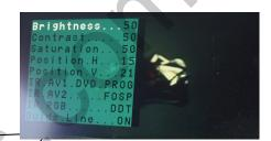
The last option: "Guide Line.....ON": the installer can set ON/OFF to enable the parking guide line, which shows the safe zone when parking.
