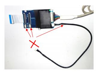
These 3 connectors pointed by red arrow should be **NOT** connected[also no connector to wire to.].
