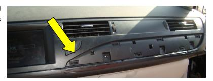
then take down the big plastic, and install the daughter board and wire for inserting video behind the monitor.
