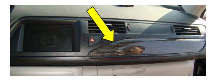
then remove the screws behind, the total plastic part can be take down, this makes the panel now shown outside.
