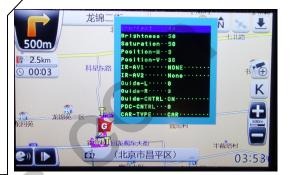
The "Guide CTRL.....ON": the installer can set ON/OFF to enable the parking guide line, which shows the safe zone when parking.
