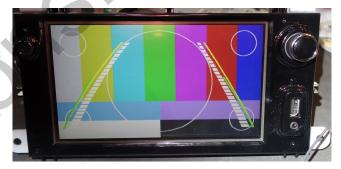
Reverse: when the driver goes to R, the can box's output [Green wire=12V], then the reverse image will be shown. And guideline can be shown if enabled by OSD.
