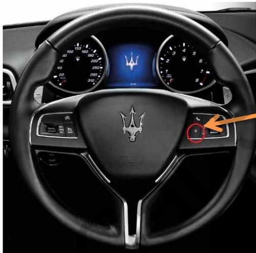
If you press long this button on steering wheel, Can switch mode
