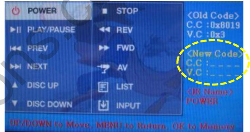
① First of all, press ◀ button on remote controller 2 seconds long. Then you can access to the FACTORY mode. And go to IR MEMORY, UTIL.
