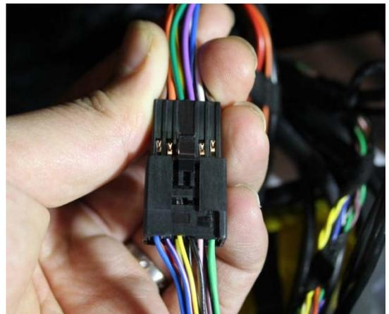
④ Please connect the cable to offered CAN IN/OUT cables.
