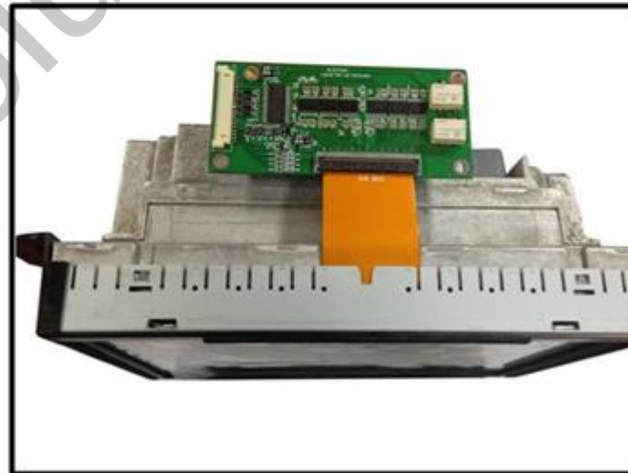
Install SUB BOARD
