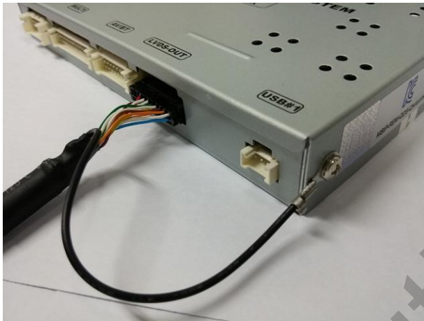
(Correct way to connect ground cable -1 )
