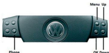
There are two main screens that can be shown on the central display (cluster), the audio- and the phone screens. Selecting these screens is possible with the 'Menu' button on the steering wheel (if available).
