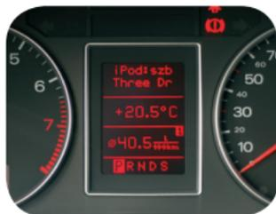
The menu of the Gateway Pro BT is displayed on the central display (cluster) on the dashboard (between the two main instruments).
