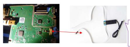
When extra navigation is installed, this daughter board can be used to switch the OEM touch panel, so the installed navigation can be touch controlled.
