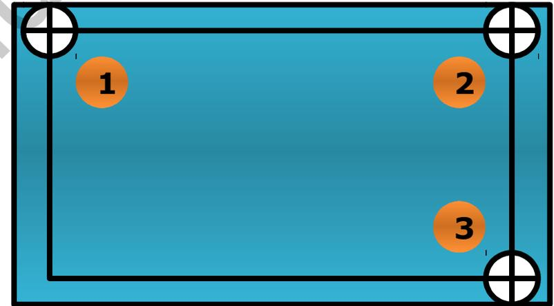
**Warning! Use stylus or not sharp object for calibration. Be sure you that you precisely match the indicated places. In case the touch screen panel is not connected, is damaged or pressed, if the connection between the touch screen panel and controller is damaged, when you enter calibration mode, "MODE" LED will blink 5 seconds and the controller will exit the calibration mode.**
