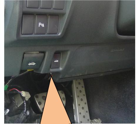
The CAN box's OBD connector should be inserted here, fixed with a type for stability.
