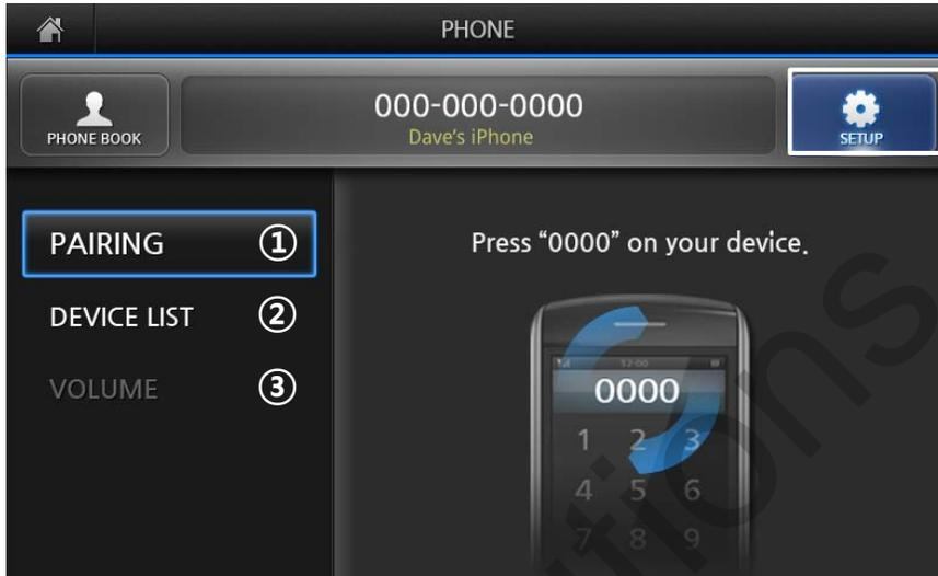
① Pairing : Press “PAIRING” button and input the password (original setting : 0000), searching device through Bluetooth and choose the phone.
