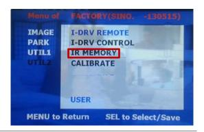
First of all, press ◀ button on remote controller 2 seconds long or press UP→DOWN→UP→MENU button in order to access Factory mode. Choose IR MEMORY on UTIL2.
