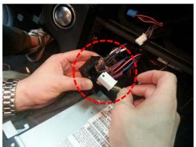
Separate white connector cable from bunch of cable behind of Audio deck
