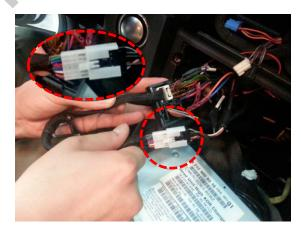
② connect provided power cable on the other side with connector as photo ①
