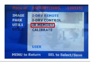
① First of all, press ■ button on remote controller 2 seconds long or press UP→DOWN→UP→MENU button in order to access Factory mode. Choose IR MEMORY on UTIL2.
