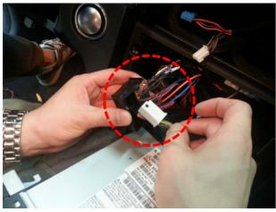
Separate white connector cable from bunch of cable behind of Audio deck
