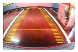
In H-POSITION, use ⊲, ▷ on remote control, to adjust parking guideline left and right.
