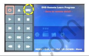
③ After register, select "SRC" button in OSD menu. Then you can see confirmation window as shown above. At the moment, (If data is saved, DVD TYPE and DTV TYPE will be changed to "USER" automatically.)
