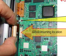
Remove this screw, then the total monitor can be taken down.
