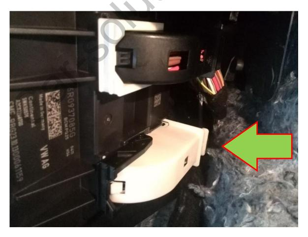
There is very little space here, so we recommend removing the driver's seat altogether before starting. Lift up the snaps and remove the connectors. A white connector will be used for installation.
