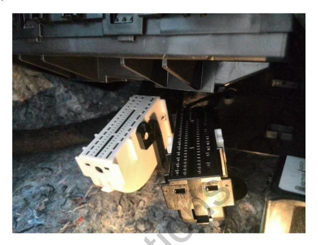
Remove the cover from the white connector. There are two snaps on the sides (from the side of the wiring).
