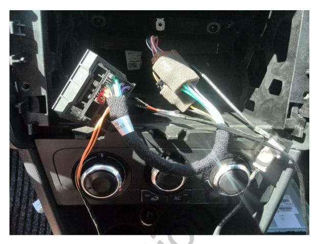
Connect to the CAN cable after checking the head unit. Move the driver's seat back, lie down near control pedals facing up and look for a **6R0 937 085 G** box. This is where the CAN cable will be wired from.
