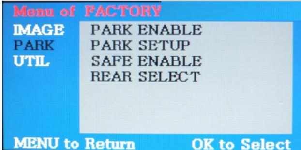
① Register the value needed on the "PARK ENABLE" as "ON" in the PARK section as shown left. **(default - ON)**
