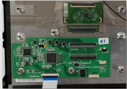
After disassembling, please place Sub board like the picture.
