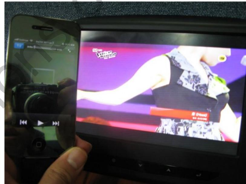
If you connect the I-pod with Qvix via I-Pod cable, you can see the media thru monitor using the apple button of the remote control
