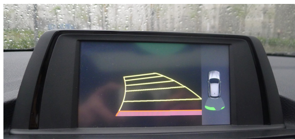
F20: Installed Camera +Guideline+OEM radar picture
