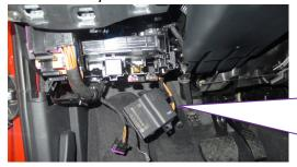
All Gateway inside an Audi looks like this, it has CAN+ Optical cable connected.
