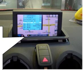
The last option: "Guide Line.....ON": the installer can set ON/OFF to enable the parking guide line, which shows the safe zone when parking.
