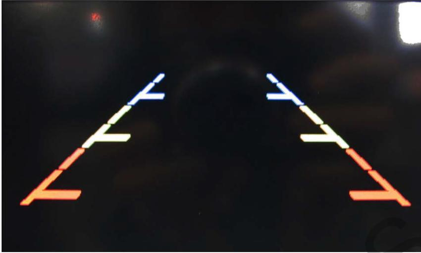
① Once you change up into rear gear, the rear parking guide line will automatically appear on the screen like the left picture.
