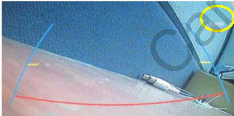
④ After you control the horizontal position with “UP”, “DOWN” button on the keypad, you can move to the vertical positioning mode after pressing “SEL” button and saving process. Once you finish that and press “SEL”, all the things will be saved. ( Adjustable between level 0 and level 255. )
