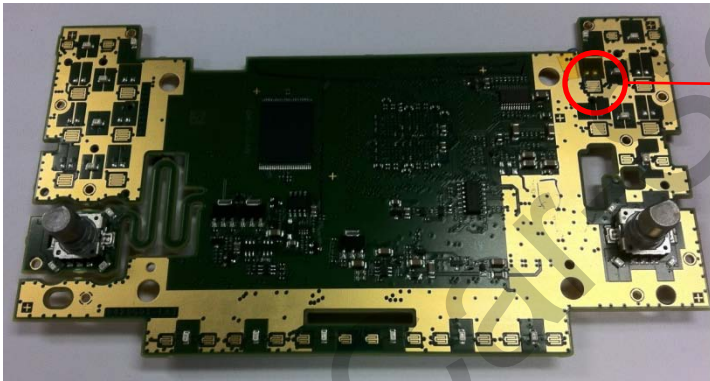
4. Soldering point – the spot near the navigation button on the LCD circuit's front (thin wire)
