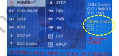
① First of all, press ◀ button on remote controller 2 seconds long. Then you can access to the FACTORY mode. And go to IR MEMORY, UTIL.
