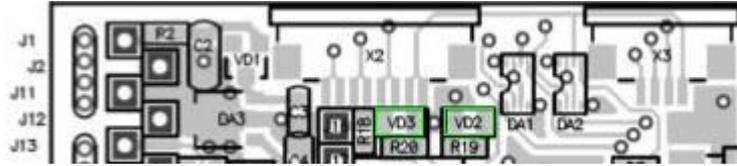
Two LEDs indicate current state or tuning phase(tuning without PC). «STATE»-VD2 (right) and «TOUCH»-VD3 (left), see figure above.
