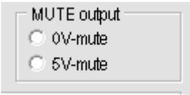
4.1. In general, this is a mute output. If NAVI has no such output, we generate it ourselves. You need to set an active level of output voltage 0V or 5V. This line is directly connected to MCU pin through 220 Ohm resistor. You may not to connect relay coil directly to this pin.
