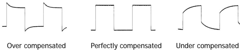
Figure 1-8 Probe Compensation
