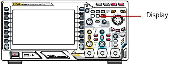
Press **Display** → **Type** to set the waveform display mode to “Vectors” or “Dots”.
