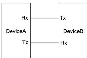
The industry standard of RS232 uses "Negative Logic", namely high level is logic "0" and low level is logic "1".
