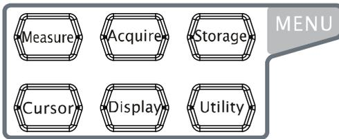
**Measure**: press this key to open the measurement setting menu. You can set the measurement setting, all measure, statistic function etc.
