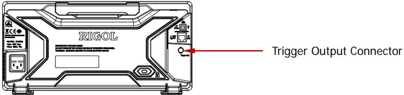
Press **Utility** → **AuxOutput** to select "TrigOut". When the oscilloscope is triggered, it will output a trigger signal determined by the current trigger setting through the **[Trigger Out]** connector.
