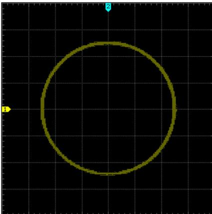
4. As shown in the figure above, the distances from the crossing points of axis and the circle to the origin of the coordinates are approximately equal. Thus, the phase deviation angle  $\theta = \pm \arcsin 1 = 90^\circ$ .
