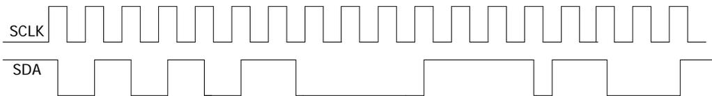
**SCLK:** sample the SDA on the clock rising edge or falling edge.
