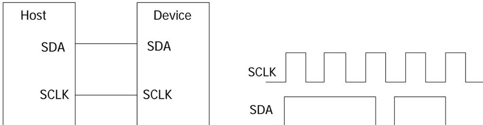
**SCLK:** sample the SDA on the clock rising edge or falling edge.
