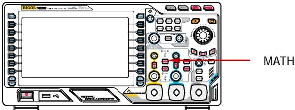
Press **MATH** → **Operate** in the vertical control area (VERTICAL) at the front panel to select the desired operation function. The result of math operation is displayed on the waveform marked with “M” on the screen.
