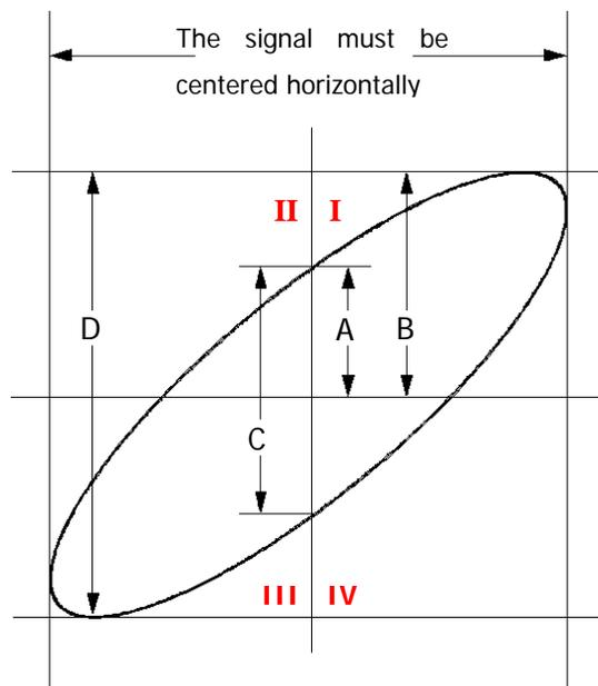
According to  $\sin\theta = A/B$  or  $C/D$  (wherein,  $\theta$  is the phase deviation angle between the two channels and the definitions of A, B, C and D are as shown in the figure above), the phase deviation angle is obtained, that is:
