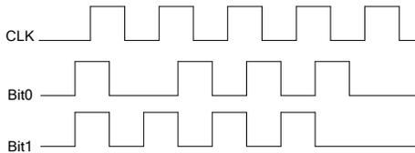
The oscilloscope will sample the channel data on the rising edge, falling edge or the rising&falling edges of the clock and judge each data point (logic "1" or logic "0") according to the preset threshold level.
