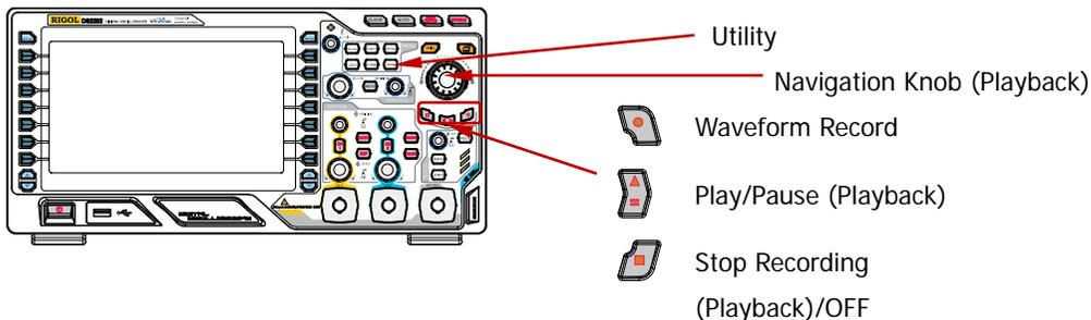
Press **Utility** → **Record** → **Mode** and use to select "Record" to open the waveform record operation menu.
