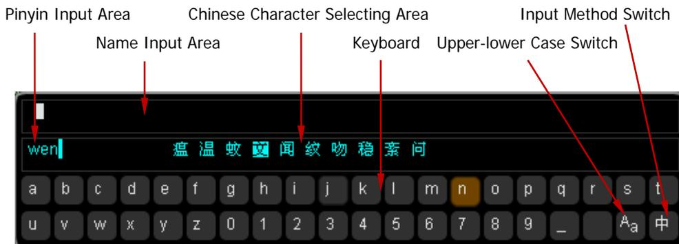
2. During the name input, you can press **Name** to select the “Name Input Area” and then press **Delete** to delete the Chinese characters on the left of the cursor one by one.
