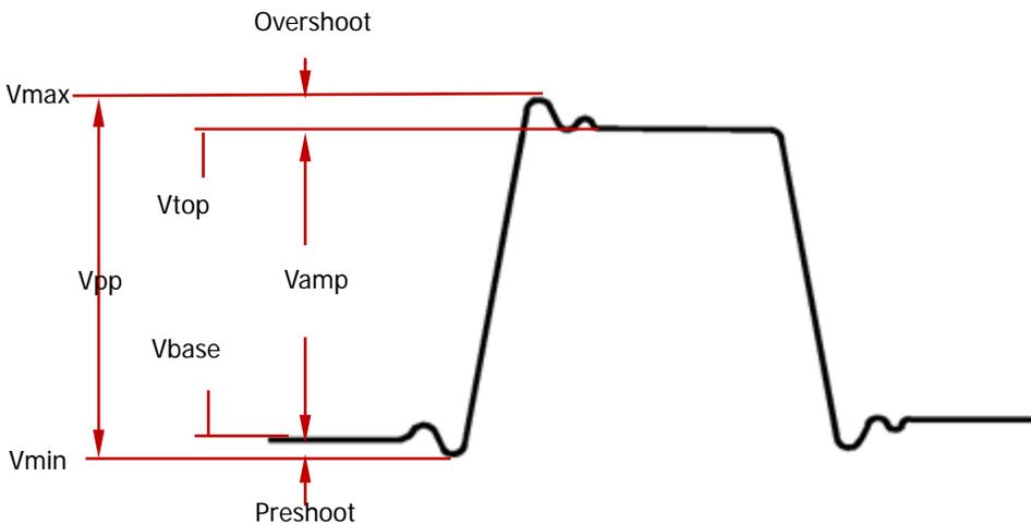
1. **Vmax**: the voltage value from the highest point of the waveform to the GND.
