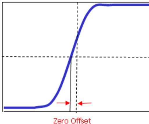
Press **CH1** → **Delay-Cal** and use
