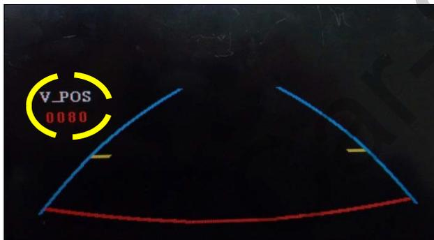
③ After adjusting horizontal position, press "OK" on the remote controller. Then you can see "V-POS" on the left of screen. At that time you can adjust vertical position of the guide line.
