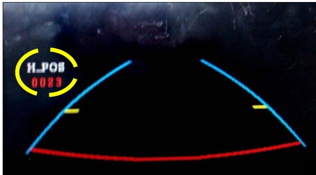
② If you get rear gear after setup, parking guide line will appear on screen as shown left. Now that you push "OK" button, you can see "H-POS" on the left of screen. Then adjust horizontal position of the guide line.
