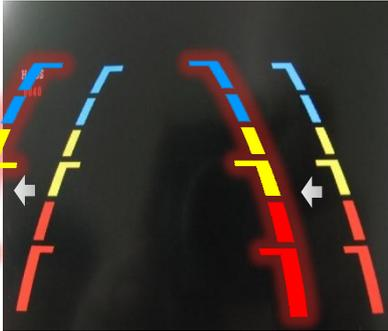
If you need to move the horizontal position, press  $\Delta$ ,  $\nabla$  buttons on the remote control.
