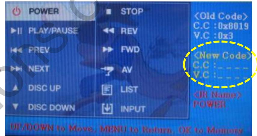
① Press ◀ button 2 seconds long on the remote control or press UP→DOWN→UP→MENU button in order for Factory Mode, select I-DRV → IR MEMORY.
