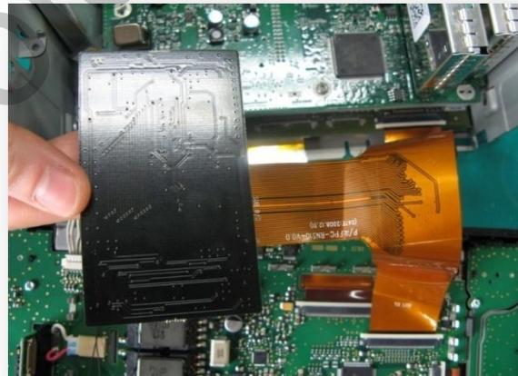
Connect the other side of FPC cable to the connector from LCD. (as shown left)
