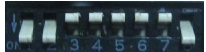
※ Please make sure to disconnect the power cable of the interface and reconnect the power cable again to apply the dip switch setting whenever changing DIP switch. Otherwise, DIP switch setting will not be applied.
