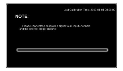
Press **Start** and the oscilloscope will start to execute the self-calibration program. Press **Exit** to give up the self-calibration operation at any time and return to the previous menu.
