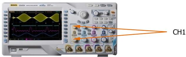
Connect a signal to the channel connector of any channel (for example, CH1) and then press **CH1** in the vertical control area (VERTICAL) at the front panel to enable CH1. At this point:
