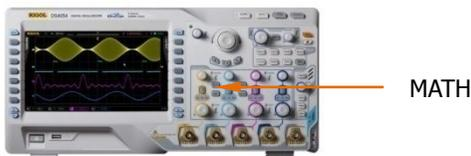
Press **MATH** → **Operate** in the vertical control area (VERTICAL) at the front panel to select the desired operation function. The result of math operation is displayed on the waveform marked with "M" on the screen.
