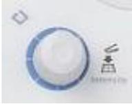
This knob can be used to adjust the value of the parameters, adjust the waveform brightness and select the desired menu (the backlight turns on during operation).
