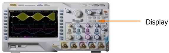
Press **Display** → **Type** to set the waveform display mode to “Vectors” or “Dots”.
