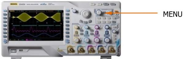
Press **MENU** in the horizontal control area (HORIZONTAL) and press **Delayed** to enable or disable delayed sweep. Note that to enable delayed sweep, the current time base mode must be "Y-T" and the "Pass/Fail test" must be disabled.
