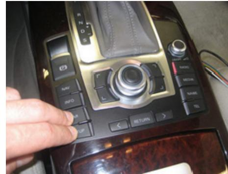
(the **SETUP** button must be pressed a bit earlier) approx. for **10 seconds** until the hidden "green" menu appears on the MMI display.
