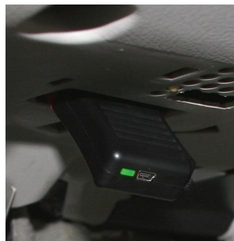
Activation procedure is **not successful** if the status signal LED is still flashing orange or goes red **after 2-3 minutes**. In this case please make sure about that the ignition was turned ON.
