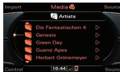
MMI's Enter function clicks into or down the menu, or plays the track once a track list is chosen. Return allows the user to navigate out or up a menu, much like the Menu button on the iPod. (The Dension Gateway MMI3 also charges the iPod / iPhone battery while it is connected)
