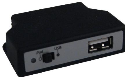
You can install our interface without having the connector port connected. In this case the USB mode will be the default mode.
