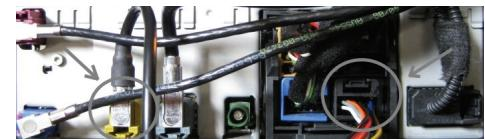
Connect the 18-pin micro-fit to the Car side of the Dension Gateway Interface and connect the round iPod connector and the connector port as well to the Gateway interface.
